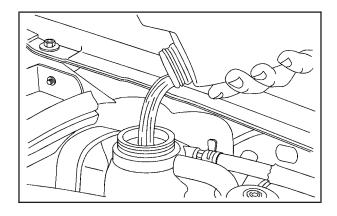
Fill the coolant surge tank with the proper mixture, to slightly above the FROID/FULL COLD line on the side of the coolant surge tank.
